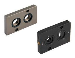
Plates to be mounted between NAMUR valve body and actuator in presence of coils thicker than the valve body (PSN type), and plates to be mounted at the speed regulator body as adapter for pipes connections (PNF type).
