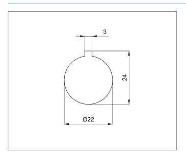
Dimensions of the hole for panel mounting. The panel must not be thicker than 6 mm.
