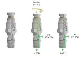
When installed in a pneumatic circuit, the pressure control sets the workingpressure of all the connected components.
